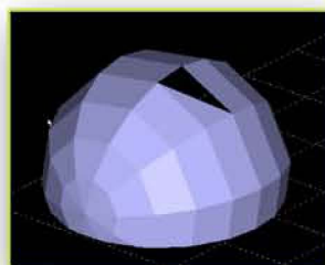
STL appears to have a missing facet
